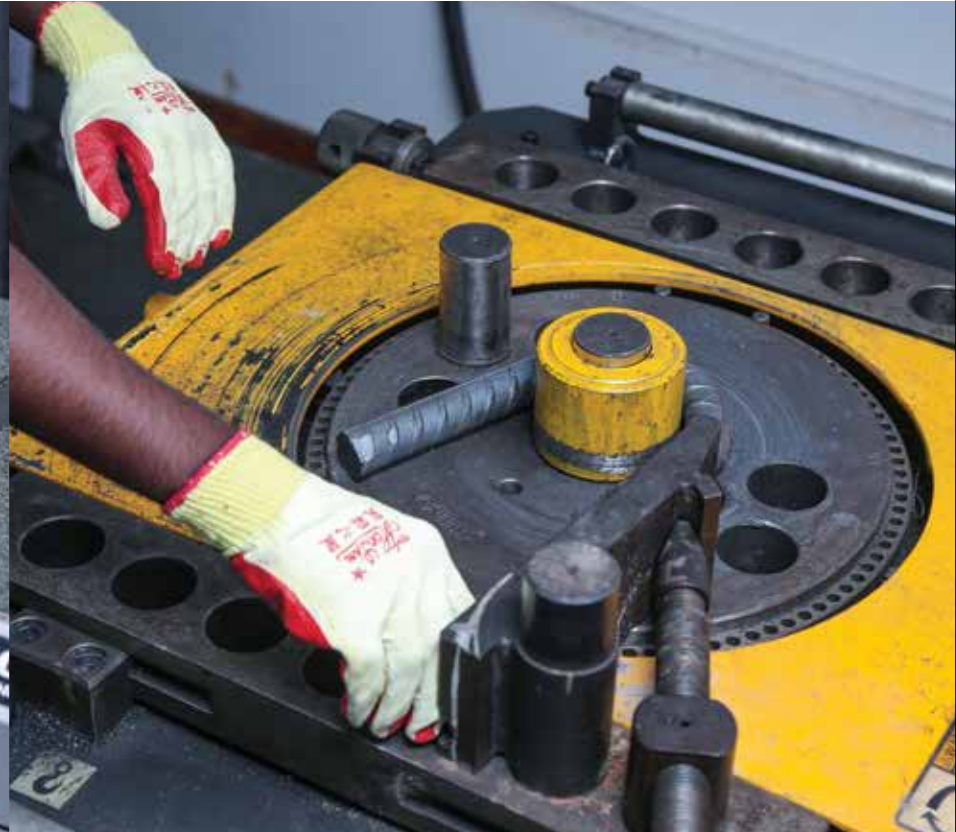
Bending and Re-bending – via fully automated equipment
